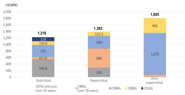
Figure 2-19 Coal-Fired Power Plants by Technology Type and Years in Operation
