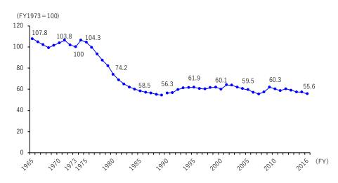
Figure 2-20 Energy Consumption Factor for Japan's Manufacturing Industries
